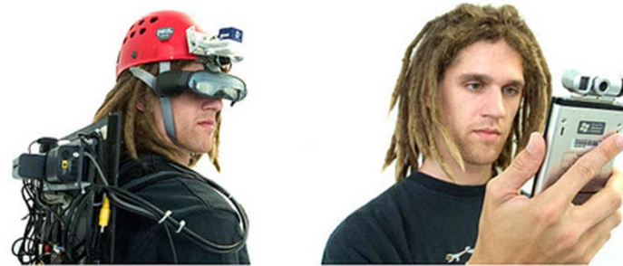
Fig. 1. A typical “backpack” setup (left) for Mobile AR versus a lightweight handheld
